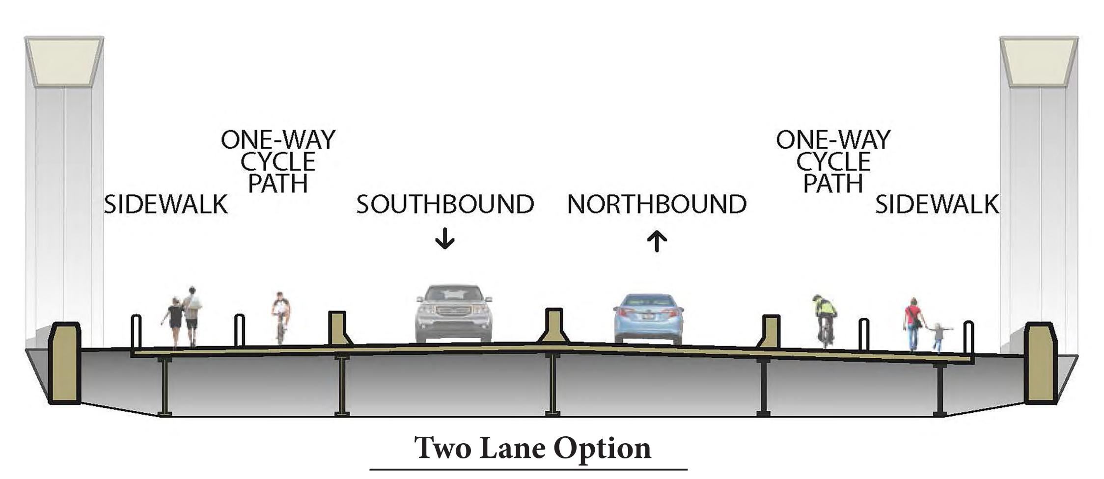
Separated one-way cycle lanes and sidewalks on both sides of bridge
